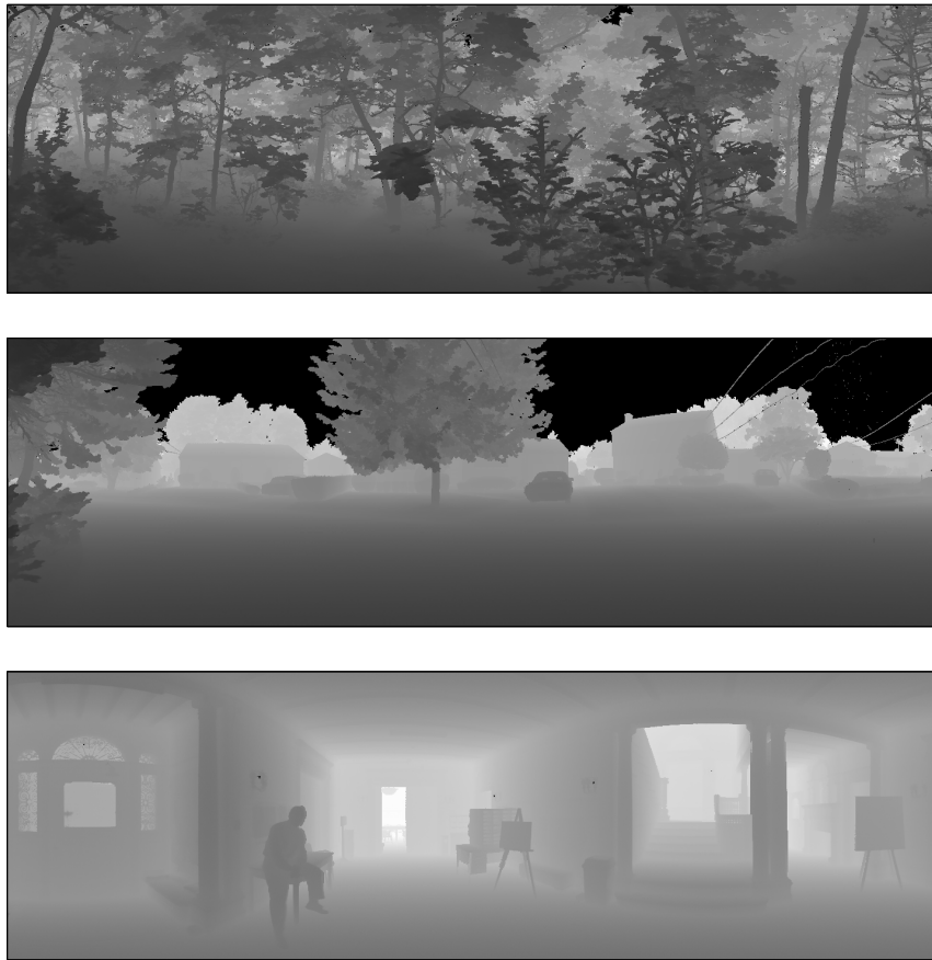
Figure 4. Samples from the Brown range image database by Huang and Lee. The gray values code for log-range values.
