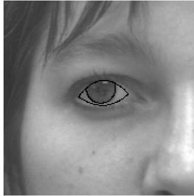
Figure 10: A flexible template of an eye, fit to a face image (from [Y-H-C]).
