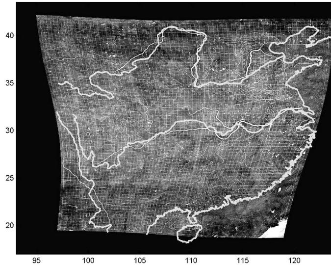
Fig. 7. The white lines and white grid are a rubbing from the original carved stone *Yujitu*. It has been warped so that 45 landmarks are at their correct positions with respect to the longitude/latitude axes. The yellow lines are the true coastline, Yellow, Yangtze and Mekong rivers. Note how far from vertical the original NS lines become.
