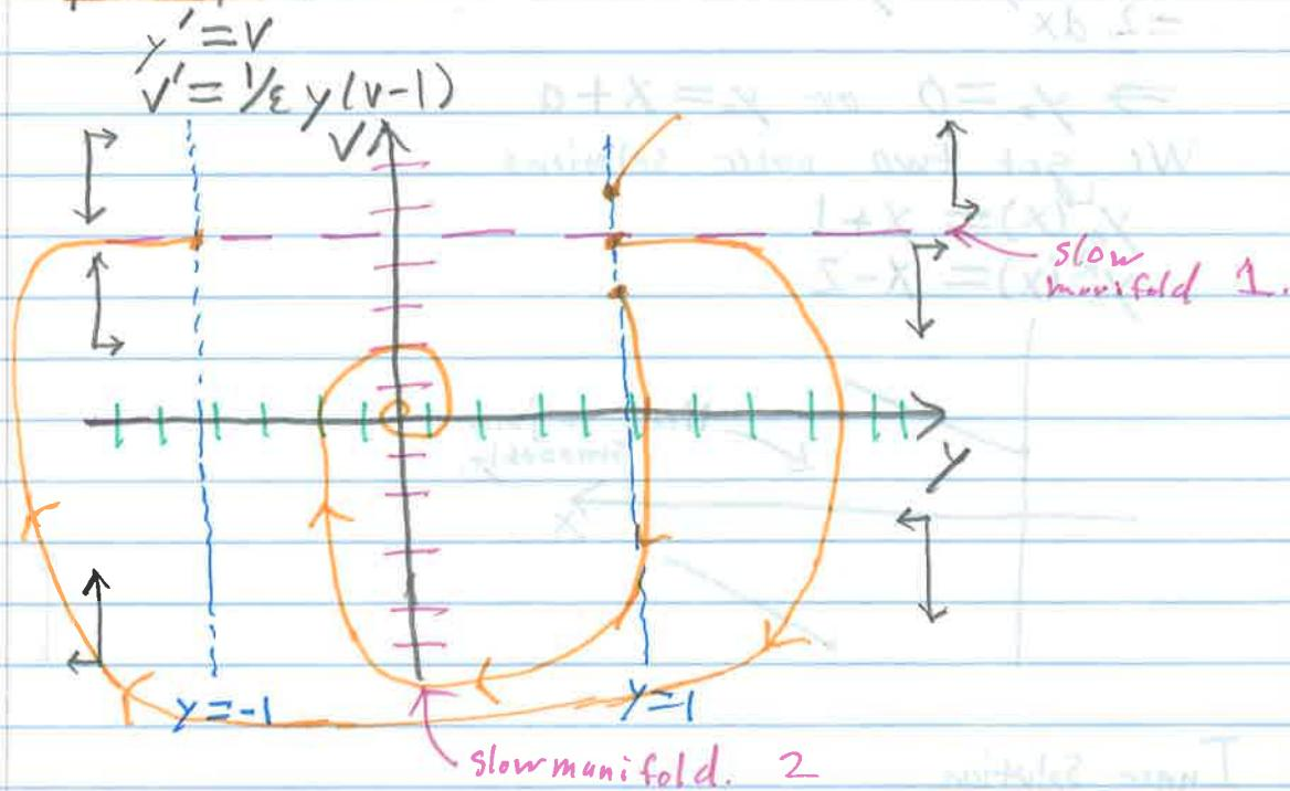
On slow manifold 1  $v=1 \Rightarrow \frac{dy}{dx}=1 \Rightarrow y=x+C$  is an exact solution. This means trajectories on the slow manifold stay on the slow manifold
