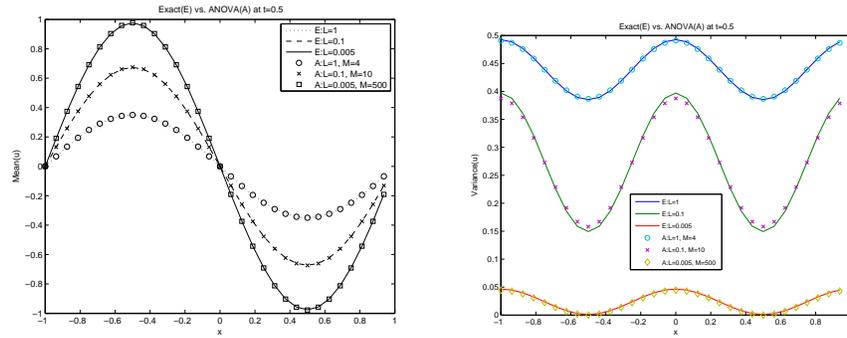
**Fig. 2** Mean solution (left) and Variance (right) using the optimum anchor point  $c_1$  for different values of the correlation length ( $L = 1, 0.1, 0.005$ ) and corresponding truncation dimension ( $\nu = 2, 2, 1$ ).
