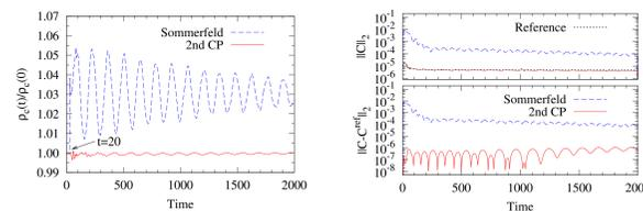
FIGURE 1: Left: radial oscillations of a compact stars' central rest-mass density in time. The outer boundary is at  $r_{\text{out}} = 20$ . Incoming constraint violation from the outer boundary perturbs the star at  $t = 20$ . Right: norm of the constraint violation in the same numerical test.
