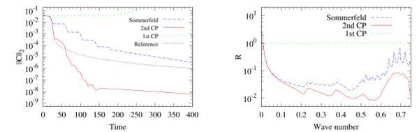
FIGURE 2: Left: Constraint violation in flat spacetime test. The 2-norm of the constraint monitor is shown in time for different BCs implemented. The same quantity for the reference simulation is shown. Right: Experimental reflection coefficient in flat spacetime test. The experimental reflection coefficient, defined in Eq. (77), is plotted versus the wave number for different BCs implemented.
