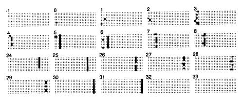
FIGURE 4. Twenty frames from a movie of a simulated synfire chain, where each vertical group represents nine neurons in an assembly, and each assembly is connected to its neighbor on the right. From [1].
