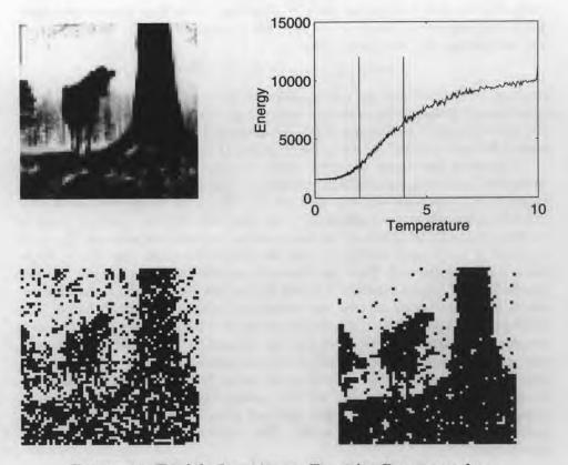
FIGURE 14. Top left: Input image. Top right: Energy as a function of temperature during the annealing process. Bottom left: An intermediate stage at a relatively high temperature in the construction of foreground/background by annealing. Bottom right: A lower temperature stage. The temperatures of two samples are marked by the vertical lines in the graph: note that they delineate the steepest part of the curve – the 'phase transition' in this example.
