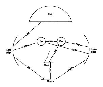
FIGURE 8. To recognize a face, one must identify its parts but allow for individual differences in the geometry of their placement. This was first modeled by Fischler and Elschlager in 1973 [13].
