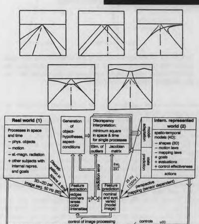
FIGURE 12. Driving by computer. Top left: The van used by E. Dickmanns. Top right: A scene in which the road is hard to locate. Middle: Fitting internal models to curved and sloping roads. Bottom: The overall Kalman-filter-like architecture of the system. © The MIT Press. E. D. Dickmanns, Expectation based dynamic scene understanding, in Active Vision, A. Blake and A. Yuille, editors, MIT Press, 1992.
