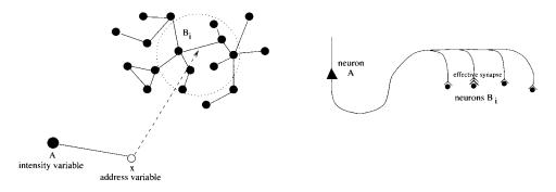
FIGURE 9. On the left, Mixed Markov models extend Markov random fields by allowing address variables which add dynamic links to the underlying graph. Address variable x can have any of the nodes  $B_i$  as its value. On the right, neural version with 'effective' synapses.
