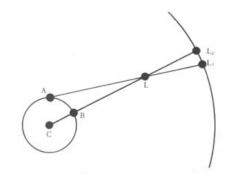
Fig. 2. The parallax of the moon: seen from point A, the position L of the moon against the sky shifts towards the horizon from where it appears at point B.
