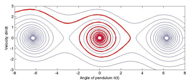
The swings which previously went over the top now can go all the way around only a few times before friction slows them down and they no longer have the speed to make it to the top. One such event is shown by the red curve; three similar events are shown in blue.
