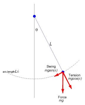
pendulum is found. If  $\theta$  is this angle, then the stretch force is  $mg \cos(\theta)$  and the swing force is  $-mg \sin(\theta)$  (note the minus sign: when  $\theta$  is positive, the force seeks to decrease  $\theta$  and thus is negative). Now as  $\theta$  is measured in radians,  $\theta$  gives arc length on a *unit* circle; as the pendulum swings in a circle of radius L, arc length along the trajectory of the pendulum is  $\theta L$ . Thus Newton's equation F=ma becomes:
