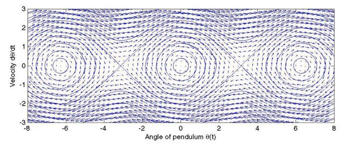
What are we looking at here? Each point in this plot corresponds to some pair of values  $(\theta, v = d\theta/dt)$ , a specification of both the position and the velocity of the pendulum. You can imagine the pendulum being released in any such state and then track what happens.
