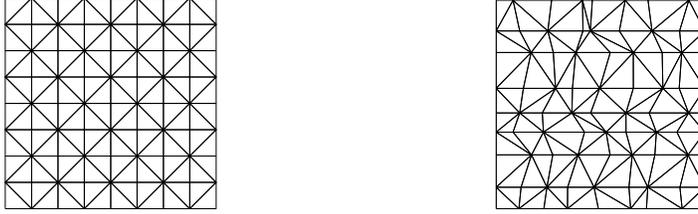
FIG. 4.1. Meshes satisfying the flow condition with respect to  $\beta = (1, 0)$ : Uniform mesh ( $h = \frac{1}{23}$ ) (left) and its nonuniform perturbation ( $\ell = 3$ ) (right).
