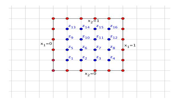
FIGURE 3. Grid, N = 4, grid points  $S_b$  are in red and  $S_I$  in blue
