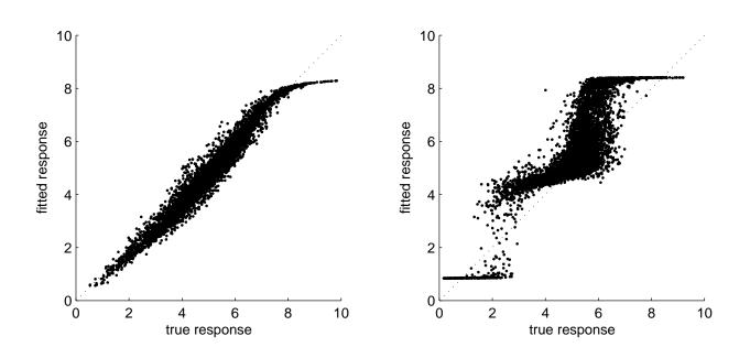
Figure 6.9: Comparison of true and fitted models on natural images. The left and right models are the same as in Figure 6.8. If the models were identical, all the points would lie on the diagonal dotted line because these plots show the mean (ideal) response, not the noisy Poisson observations. The estimated rectifier in the model on the right was wavy, unlike the true rectifier.
