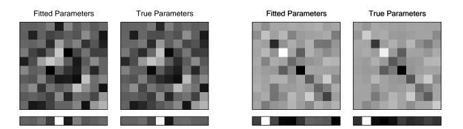
Figure 6.8: Fitted versus true parameters in the quadratic model. The upper, square images show the A matrices in the quadratic form. The lower, rectangular images show the B vectors. The left two plots are from the SFA unit used in the text. The right two are from another quadratic SFA unit. The true parameters have been projected into the 10-dimensional PCA space for easy comparison with the fitted parameters.
